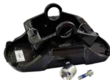
**KOMPLET NAPRAWCZY NÓG PODPOROWYCH JOST MODUŁ B /****MOUNTING KIT FOR LANDING GEAR MODUL B**
